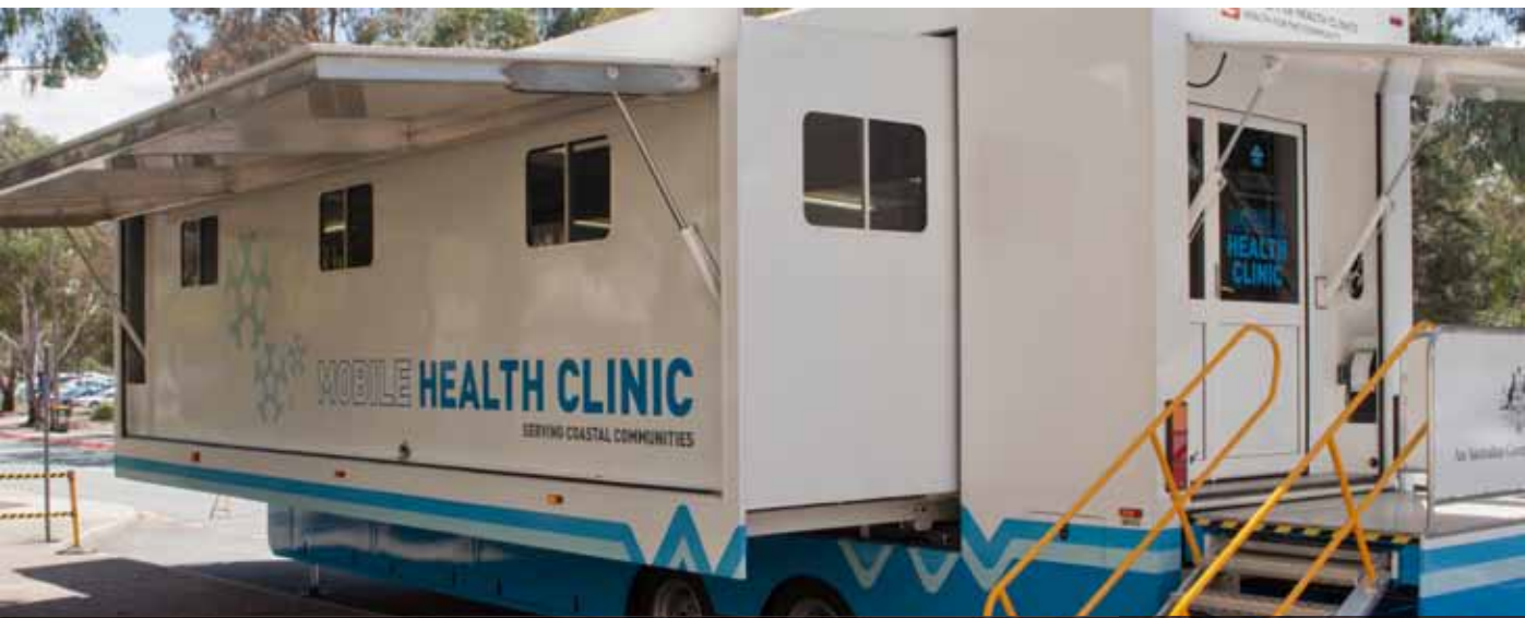
The faculty's new mobile clinic is 14 metres long and expands to 16.5 metres long and 7.5 metres wide when operational. It weighs 20 tonnes and contains stretchers, consultation rooms, classroom space, kitchen, storage, office, lounge and an electric hydraulic wheelchair lift. It will initially provide services in physiotherapy, nutrition and dietetics. It was formally launched by Andrew Leigh MP.
